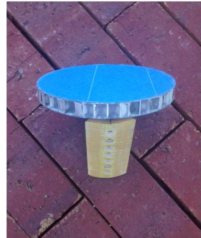
Master Power Switch Block And Honeycomb Aluminum/Fiberglass Bulkhead
