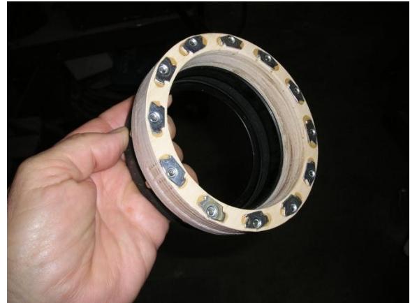
Plywood Aft Centering Ring with Aero Pack Motor Retainer
