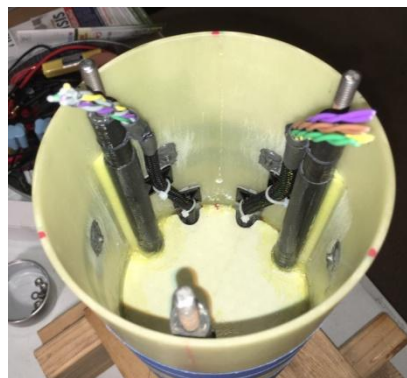
Altimeter area with routed Master Power and aft end cap terminal block cables
