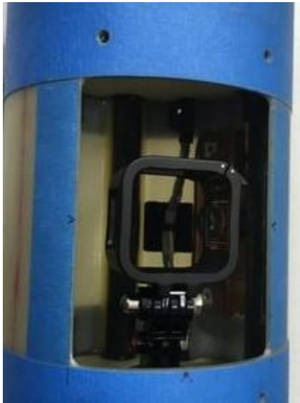
GoPro Mount (Power Switches and Aft End Cap Cable in Background)
