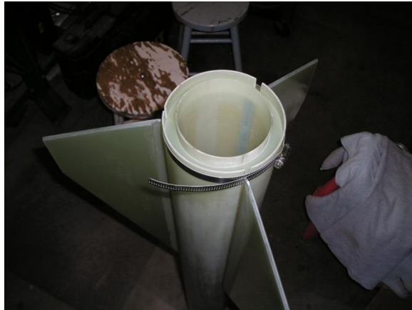
Temporary Clamping for Forward Centering Ring Bonding
