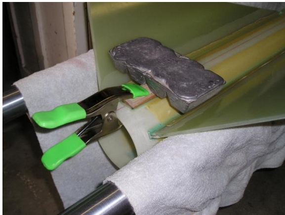
Bonding the Backing Block
