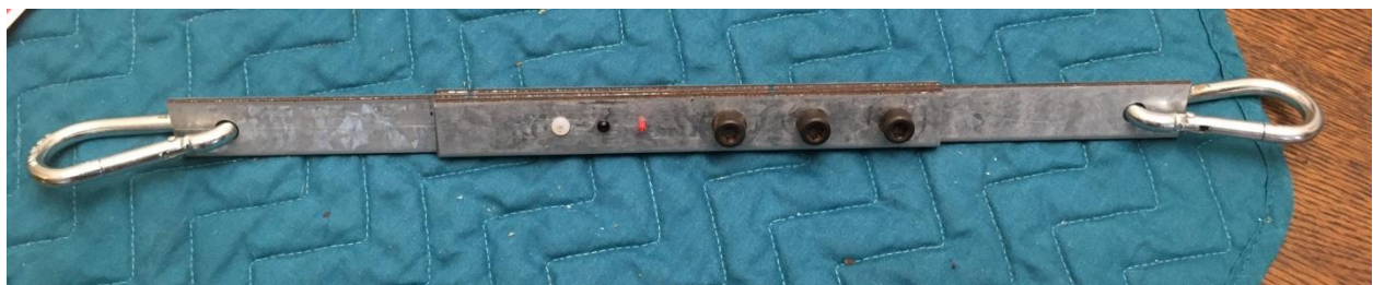
"Shear-Pin" Test Fixture (Three pins shown for clarity... not for actual testing)
