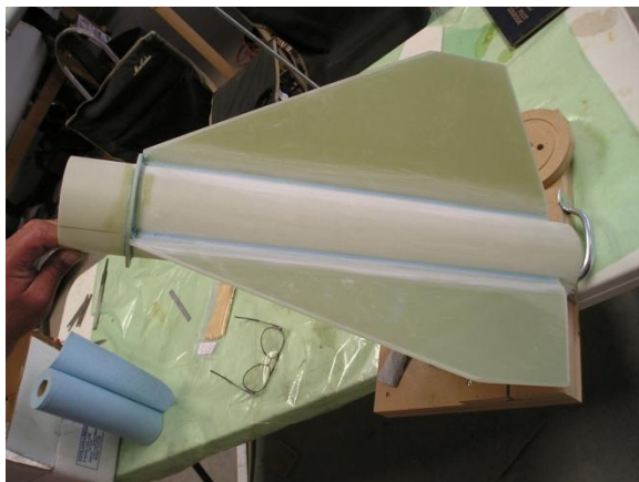
Kevlar Tape Reinforcement to Fin Can
